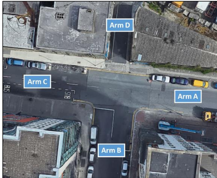
Figure 7.4: Junction 6 Existing Priority Controlled Junction Layout
